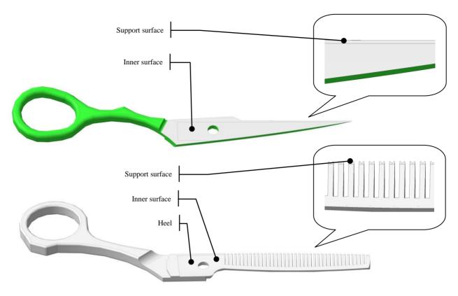
Figure 3. Scissors geometry
