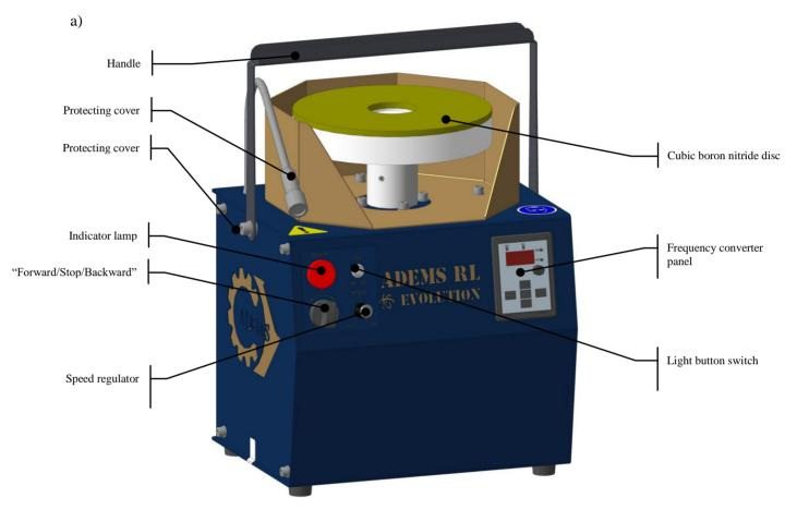
Figure 2. ADEMS RL Evolution sharpening machine
